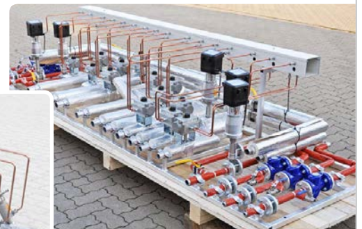
Steam packages for tire curing presses
